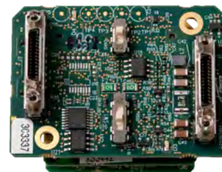
iPORT CL-U3-IND External Frame Grabber OEM Board Set (903-0020) for Camera Link Medium Mode
