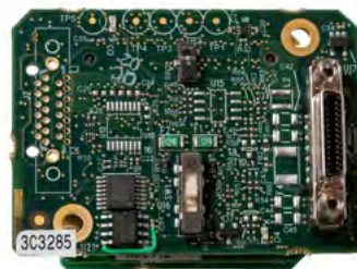
iPORT CL-U3-IND External Frame Grabber OEM Board Set (903-0019) for Camera Link Base Mode
